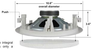
Before mounting the **40AE** speaker, push the four mounting brackets to pop off the grill as shown in the diagram.
